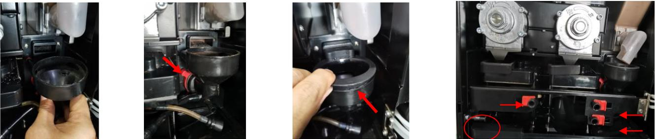
Push the body of the mixer to the bottom; Finger counterclockwise rotation fixed circle, until the rotation is not moving; The mixer cover is inserted into the steam cover and flattened; Pull out the sheet metal fastener, and install the sheet metal fastener; Install the fixing buckle of the outlet pair adapter; The nozzle is in position, and the mixer is installed and rinsed.
