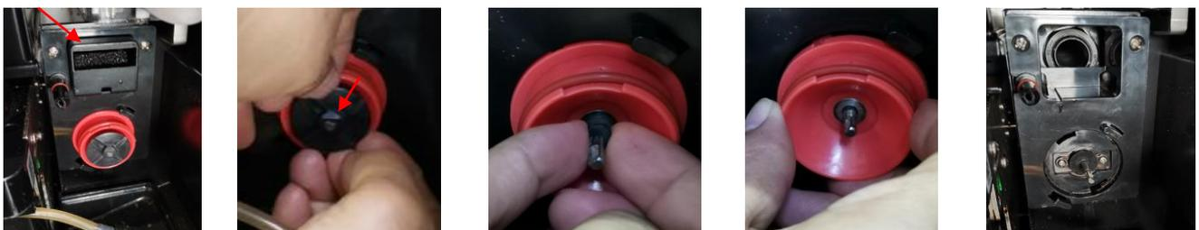
Pull out steam cap; Pull out the mixed impeller with fingers; Take out the V-ring seal; Rotate the gland clockwise and pull out; Wipe the mixer holder with a towel or wipes containing 75% alcohol;
