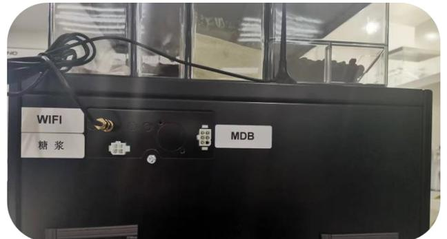
Remove the antenna from the inside of the machine and attach it to the interface at the back of the machine.
