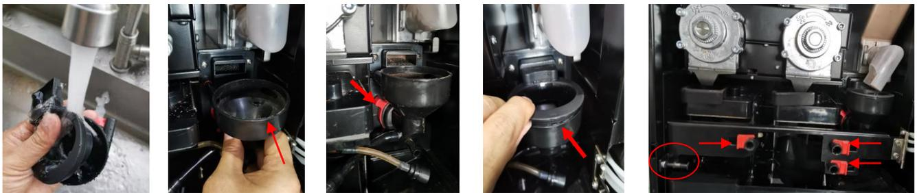
Put the rinsed mixer back into the machine: push the body of the mixer to the bottom; The finger counterclockwise rotation fixed circle, until the rotation is not moving; The mixer cover is inserted into the steam cover and flattened; Pull out the sheet metal fastener, and install the sheet metal fastener; The nozzle is fixed to the plug and adapter buckle back; The nozzle is in position, and the disassembly and washing of the mixer is completed.
