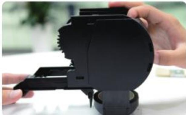
Pull out the slag scraper slider
