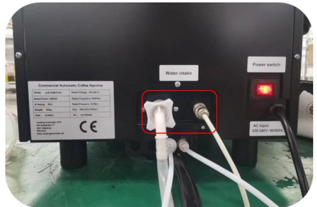
The other end of the submersible pump is connected with the machine water inlet and the submersible pump power connector.
