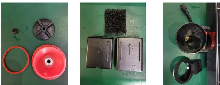
Clean mixer body, gland, V, O seal ring, mixing impeller, mixer steam inlet upper and lower cover; V, O ring regularly check whether damage, If damaged, replace it in time.
