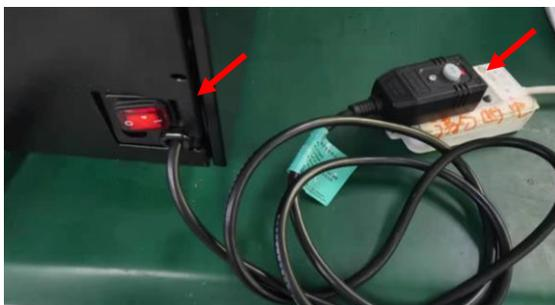
Insert the male end of the power cord of the coffee machine into the socket of the power supply; press the power switch on the back of the machine; it takes about 5 minutes for the machine to cold start.
