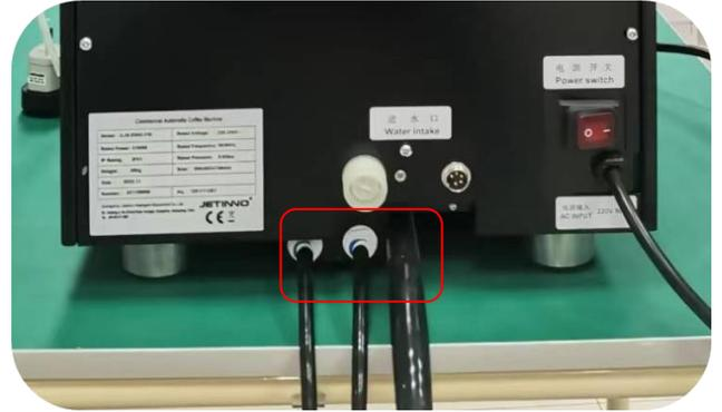
As shown in the figure above, insert the waste water pipe into the coffee machine waste water outlet connector; The silicone tube is inserted into the waste milk outlet joint; Place the outlet of the waste water pipe and waste milk pipe above the waste water bucket or waste tank.
