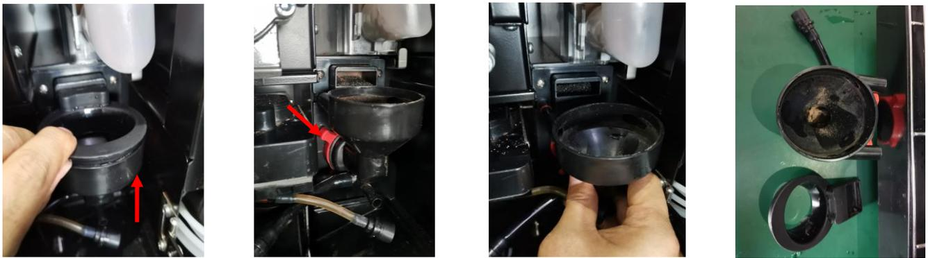
Lift out the mixer cover; Turn the fixing ring clockwise with your finger, unlock the latch, hold the mixer and pull out; Place the removed body and cover of the mixer under running water and rinse.
