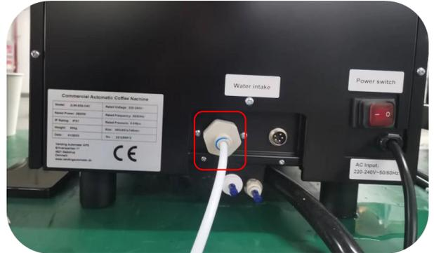
Connect the interface at the water inlet, insert the direct drinking pipe into the interface of the quick connector, install the blue buckle back, and open the water inlet valve switch.
