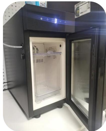
Insert the milk tube at one end of the coffee machine into the interface on the left side of the refrigerator, straighten the milk tube, and move the refrigerator to the level of the coffee machine cabinet.
