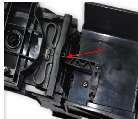
3. Pull out the pipe connector of the filter brewer downward; Connecting rod convex column (crank) to the filter brewer slag scraper middle notch position;
