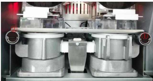
Two grinders with two adjustment positions ① and ② on the grinder; adjust the coarseness of the grind according to the screen print (the right side grinder is clockwise to adjust the fineness and counterclockwise to adjust the coarseness of the grind; the left side grinder is clockwise to adjust the coarseness and counterclockwise to adjust the fineness of the grind).
