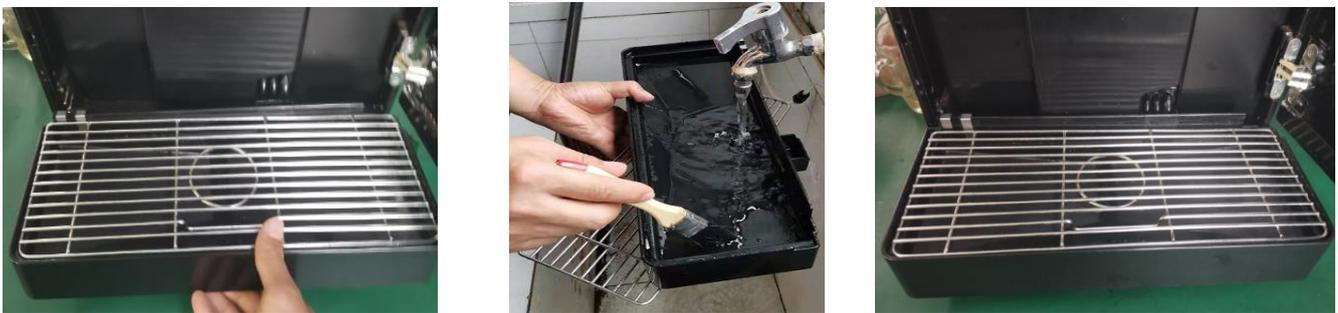
Turn the key clockwise to unlock the door; Press the metal pin on the top of the door and open the door; Take out the drip tray and the mesh set, rinse them and clean them with a brush or a towel, then install it back. Close the machine door.
