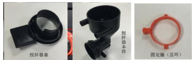
Pull out the mixer silicone tube; Rotate the red fixing ring clockwise, and after unlock, pull out the Mixer outside; and remove the upper and lower covers; Clean the mixer cover, mixer body, pressure ring, and upper and lower covers, wipe them dry and put them back.
