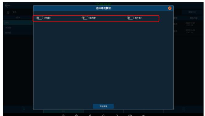
Login backend interface-cleaning Tab-Module-Machine-Manual cleaning-One-click cleaning/Quick cleaning. One-click cleaning is cleaning whole water system including tubes one time. Quick cleaning is cleaning selected module on the pop-up menu.
