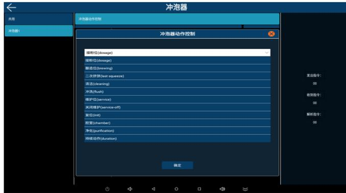
The brewer inlet pipe is inserted into the quick connector to the bottom; Click on the lower right corner of the screen and click on [Settings] -> [Brewer] -> [Brewer Action Control] -> [init]; When the brewer completes the action, abnormal standby will appear in the middle of the screen.
