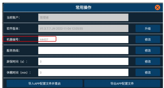
Input the capacity of each canister and do calibration test (refer to sections 6.2 and 6.3); Click "More Operations", find the machine number on the nameplate (the last five digits of the machine number), and enter the machine number in the "machine number" position.
