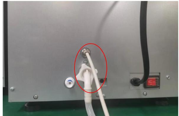
The other end of the submersible pump is connected with the machine water inlet and the power connector of the submersible pump.
