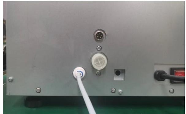
Take off the blue buckle, press the elastic surface of the quick connector, pull out the stopper, insert the direct drinking water pipe into the interface of the quick connector, reinstall the blue buckle, and open the water inlet valve switch.
