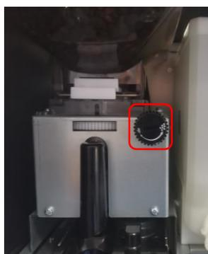
To adjust the coarseness and fineness of the grinder according to the silkscreen layout.
