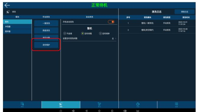
Pull out the water tray, turn on the drain switch, install the water tray, enter the password into the background, disconnect the water source connected to the machine or unplug the pump power plug, click the lower right corner [cleaning], click [empty boiler]. After waiting for five minutes, close the door and unplug the machine.
