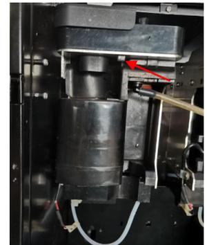
The two guide wheels at the bottom of the brewer should correspond to the two guide grooves on the brewer drive. The two guide wheels of the brewer should be put into the guide grooves in the
