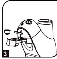
Open the handle and change for a new capsule. Press any volume key back to stand by.
