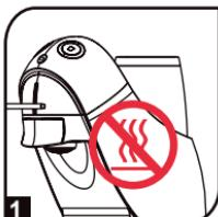
The machine shuts down both boiler and pump when there is an NTC error.
