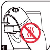
When the machine has worked/brewed continuously for 2 liters of water, the system will stop working and give a warning (if machine hasn't worked/ brewed continuously or pausing more than 5 minutes, machine start recount).
