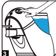
Press any volume key to recover stanby fill up the tank, press any volume key again to start the machine.
